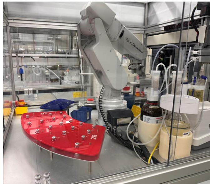
Automated Karl-Fisher for moisture measurements
