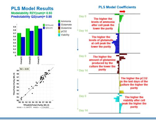
Quality attribute estimator using traditional process sensing and in-line Raman.
