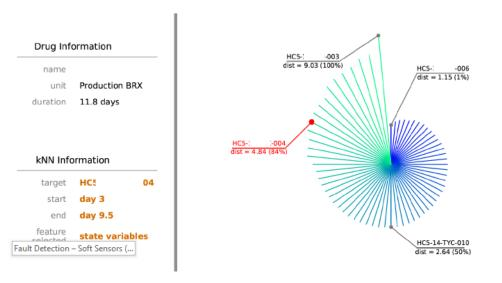
Similarity analysis can be used to calculate the distance/deviation of a batch to the historical average. Therefore, the tool can also help select representative or 'golden' batches.
