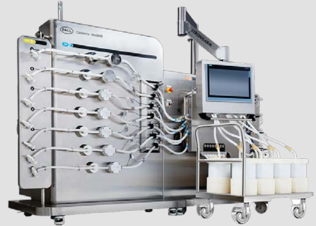
Chromatography skids with single-use flow paths and pre-packed disposable columns Source: GE HealthCare and PALL
