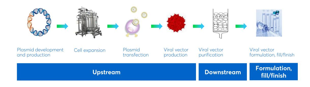
Manufacturing of AAVs is a complex process that requires several upstream, downstream, and fill/finish operations
