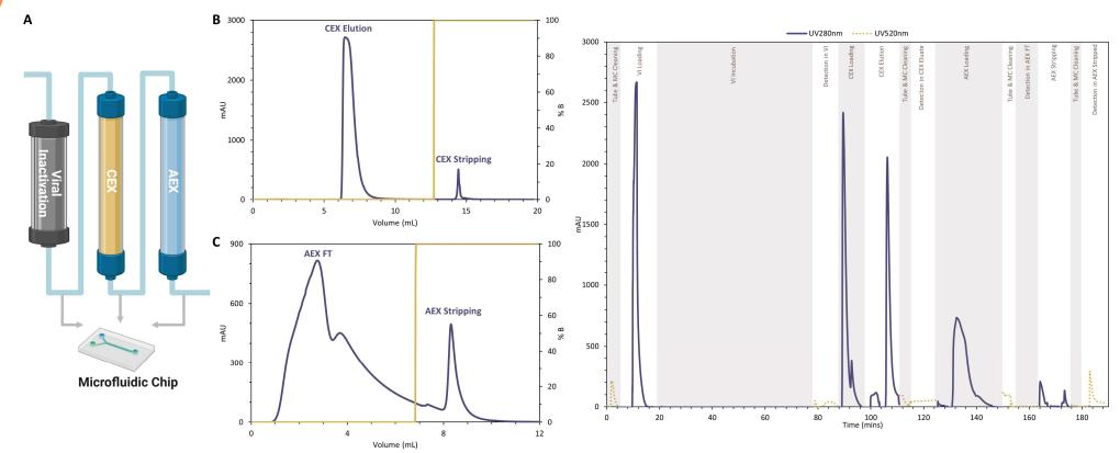
Schematic representation of integrated downstream processing (left) and chromatographic profile with aggregate detection (right)
