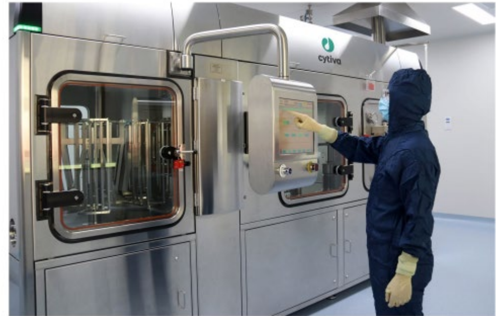
SA25 Aseptic Filling Workcell installed in a Grade C Cleanroom
