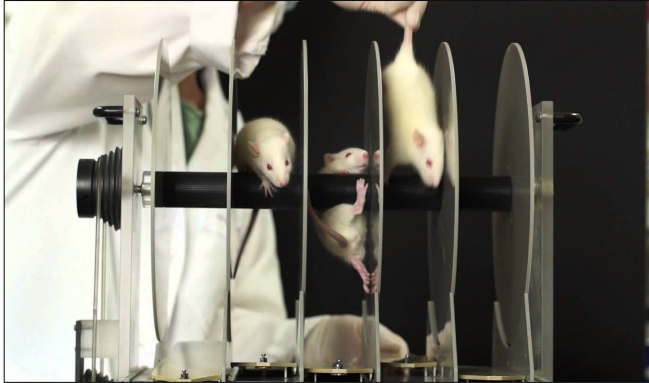
Measuring latency to fall from an accelerating, spinning rotarod
