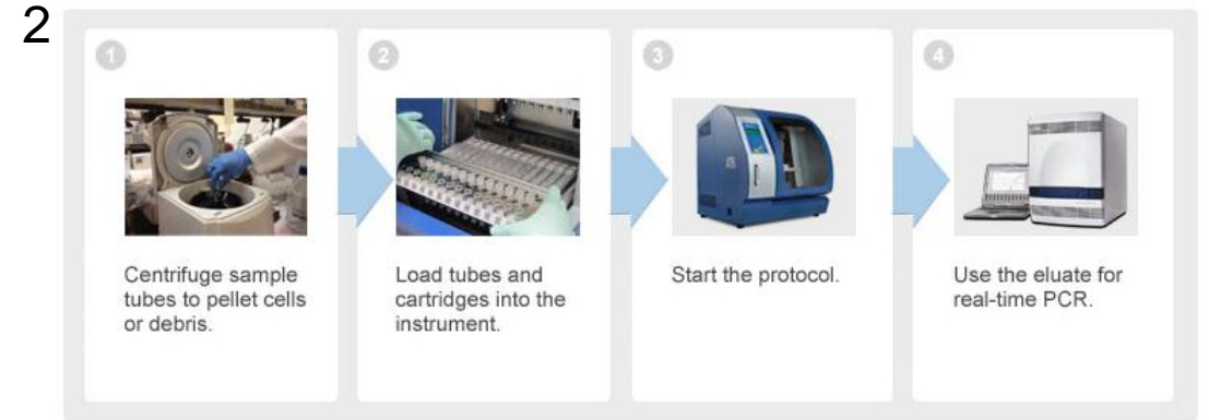
Figure 3. One-hour workflow for the AutoMate Express™ system.
