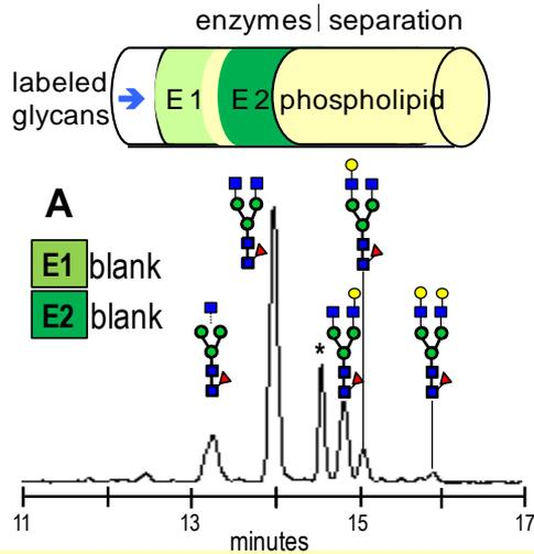
The integration of enzymes in series in a capillary for the hydrolysis and separation of glycans from Trastuzumab.
