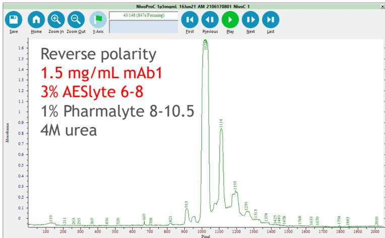
Peak identification of collected fractions using analytical iCIEF
