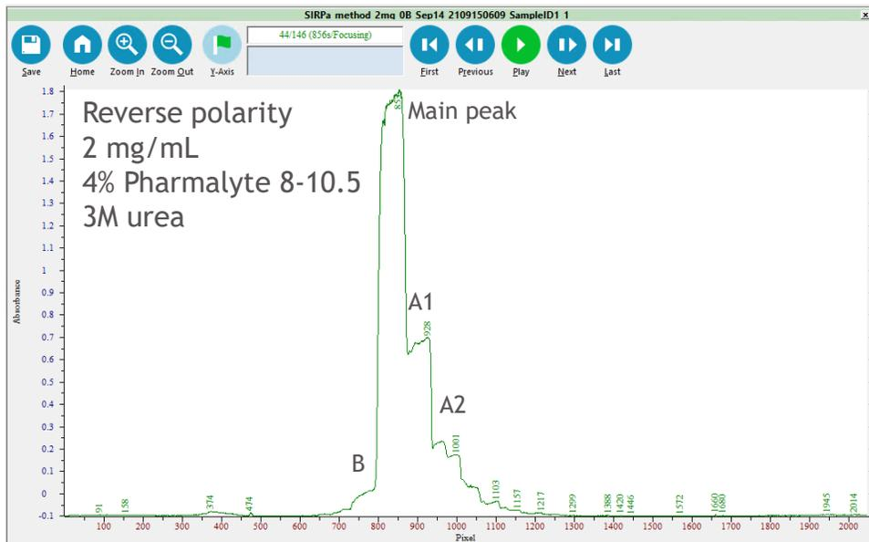
Peak identification of collected fractions using analytical iCIEF system
