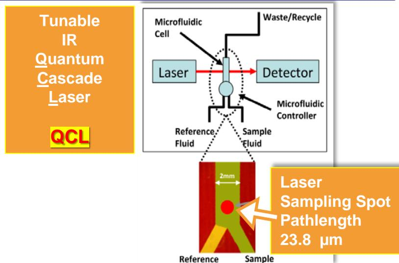
MM-IR made room temp detector possible by brighter laser QCL
