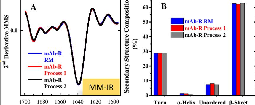
HOS comparability study of mAb-R DS from 2 different manufacturing processes analyzed side-by-side with RM (A) Overlaid 2<sup>nd</sup> derivative MM-IR spectra (at 1 mg/mL); (B) Secondary structure composition (%)
