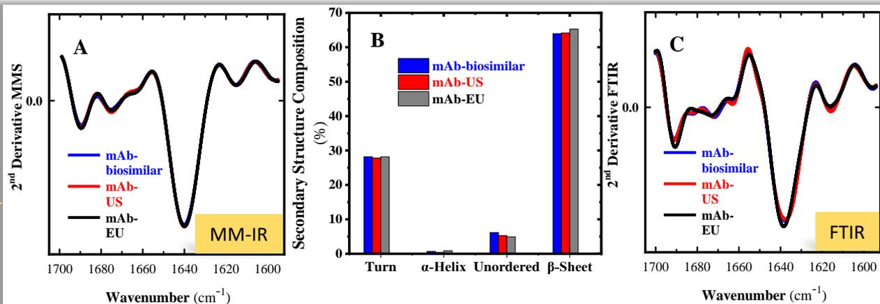
HOS similarity study of mAb-biosimilar MM-IR and FTIR (A) Overlaid 2<sup>nd</sup> derivative MM-IR spectra (at 1 mg/mL). The biosimilar is **99.1%** similar in structure (using **spectral similarity** via AO calculation) when compared to both US & EU originator products. (B) Secondary structure composition (%); (C) Overlaid 2<sup>nd</sup> derivative FTIR spectra (at 10 mg/mL)
