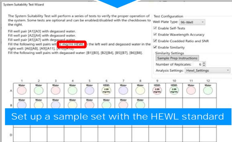
Set up a sample set with the HEWL standard
